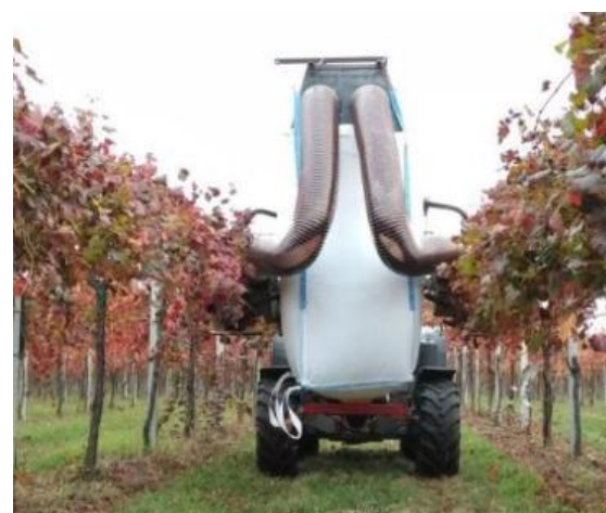
Figure 6: 1 st version of the vine leaves harvesting apparatus during operation
