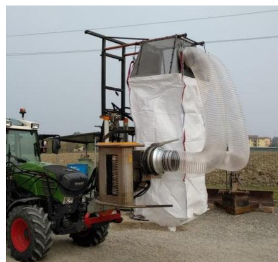
Figure 5: 1 st version of the vine leaves harvesting apparatus
